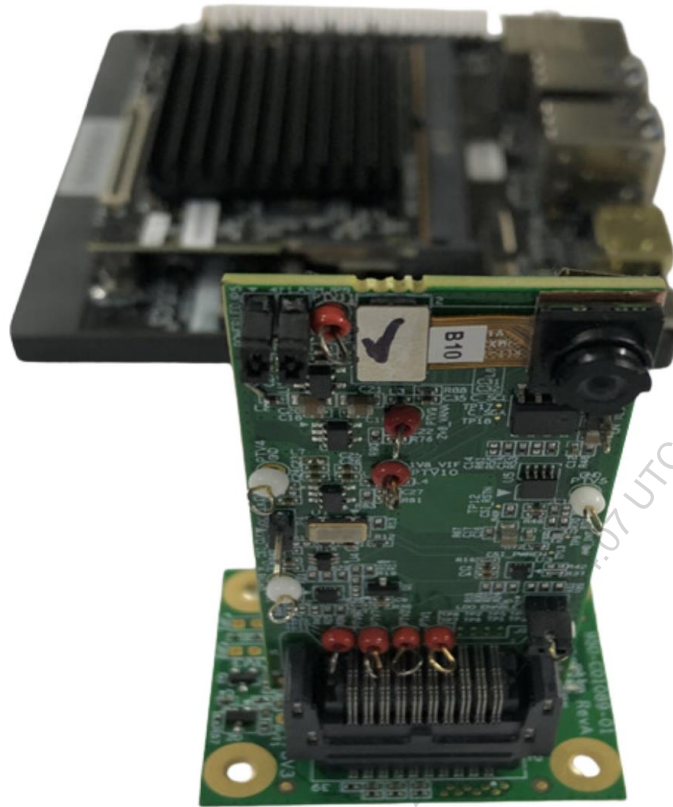
Figure 9. Connector connection with IMX258 module adapter
