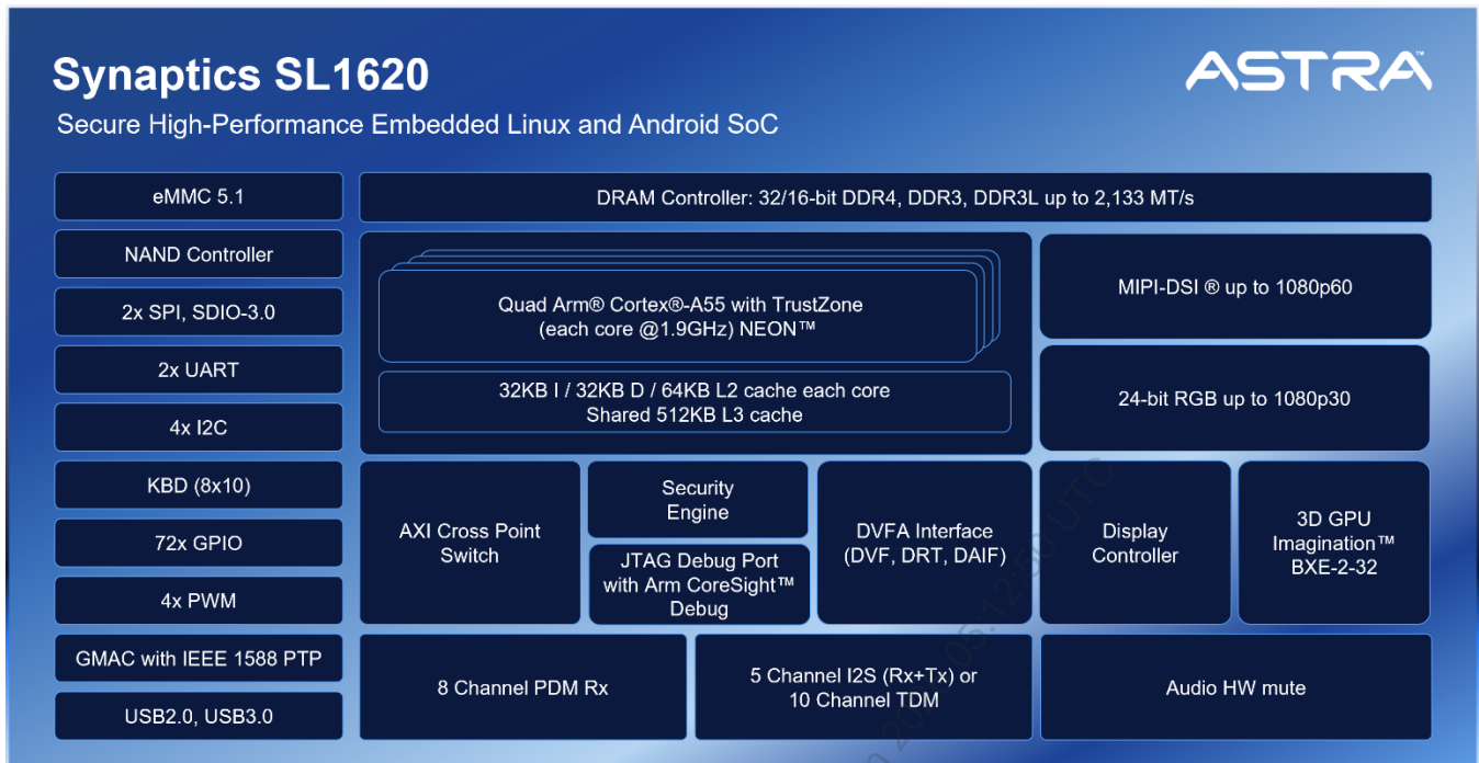
Figure 1. Astra SL1620 high-level block diagram
